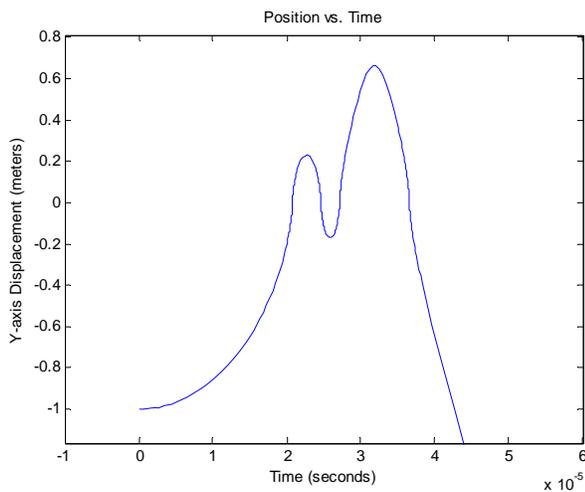
**FIGURE 4b-** Xenon Ion Displacement v. Time when the magnitudes of the positively and negatively charged plates are equal. The atom oscillates in and out of the rings before being accelerated back into the engine.
