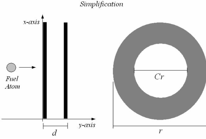
FIGURE 2 – Diagram of Simplified Electrostatic Ion Engine with Variables and Coordinate System. The region circled in Figure 1 is simplified above for our model. Two charged rings, representing a small section of the grid shown in Figure 1, accelerate one fuel atom through their center and out into space.
