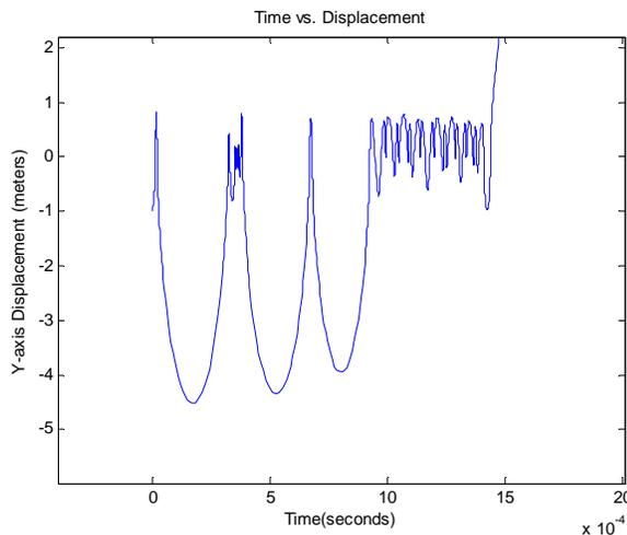
**FIGURE 4c-** Xenon Ion Displacement v. Time when the negatively-charged plate is stronger than the positively charged plate. The atom oscillates in and out of the rings before being accelerated out of the engine.
