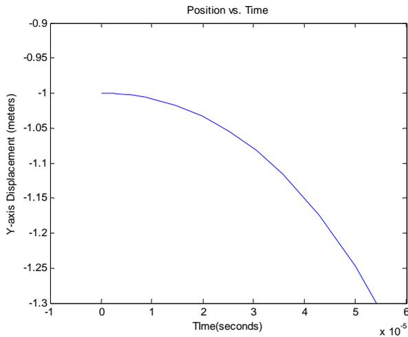
**FIGURE 4a-** Xenon Ion Displacement v. Time when the positively charged plate is greater than the negatively charged plate. The atom is simply repelled by the large positive field. The negatively charged plate is at  $y=0$  and the positively charged plate is at  $y=1$ .
