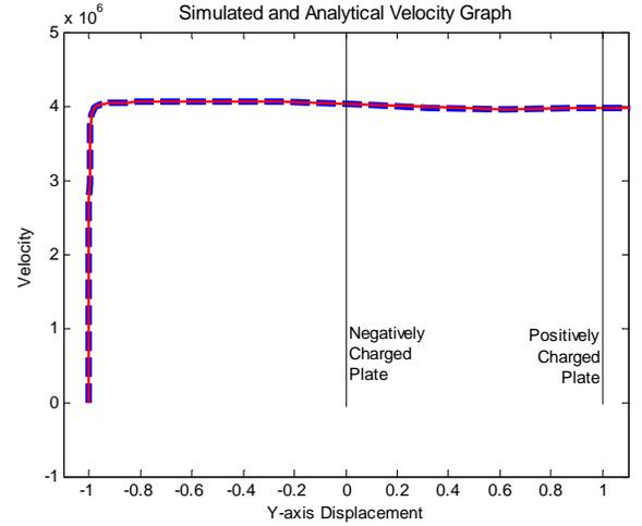
FIGURE 3 – Particle Analytical and Numerical Velocity versus Y-Axis Displacement. Red line shows numerical (i.e. simulation) solution and thicker blue line shows the analytical solution. The ion was given no initial velocity and the plates were given equal and opposite charges.
